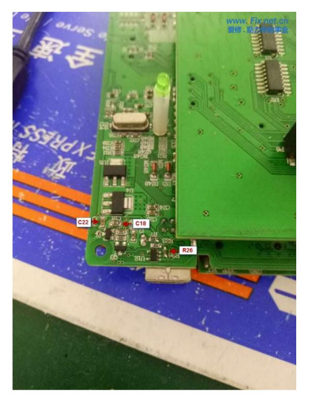
Notes : If can' t find the capacitor with patch for the C18/C22, then use the electrolytic capacitor parallel (pay attention to the polarity) connected with 47uF-100uF/16v.
